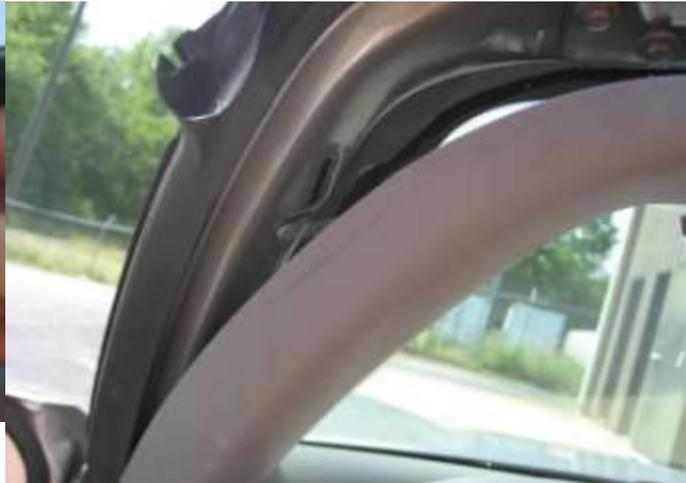
Again using your fingers, Gently pull the A-pillar around the roof pin guide and downward. There are two metal Spring Clips on the more vertical area of the pillar. **USE CAUTION...**There are several electrical harness and connectors that will need to be disconnected . The stock tweeter and possibly the On-Star microphone. Please disconnect these at this time.
