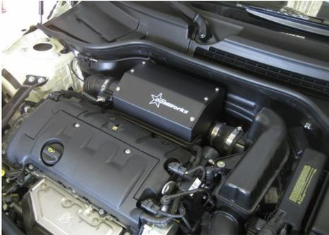
This DDMWorks Cold Air Intake improves your MINI Cooper by supplying your engine with cold air for it to breathe in through a free flowing filter.
